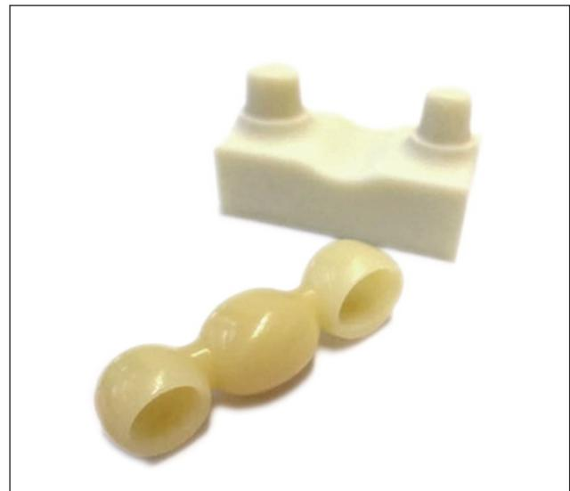
Fig. 8: Test specimen geometry for the chewing simulation
