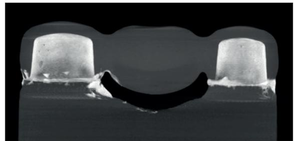
Figure 9:  $\mu$ CT image of the cemented bridge after chewing simulation
