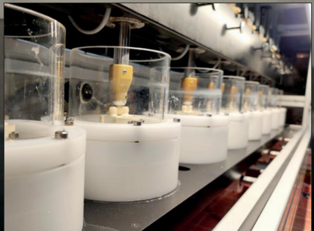
Fig. 6 and 7: Experimental setup of the chewing simulation for long-term temporary bridges
