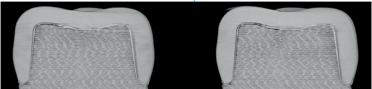
Fig. 11: Comparative  $\mu$ CT image (sectional view) of a cemented crown before (left) and after (right) the chewing simulation
