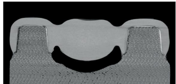
Figure 10:  $\mu$ CT image (sectional view) of the cemented bridge after the chewing simulation
