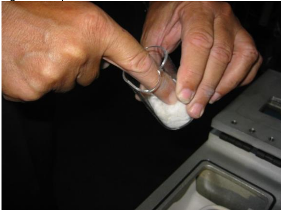
Figure 16: quartz fleece in inductor shield
