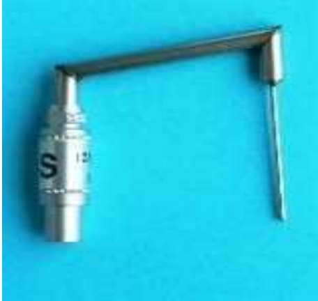
Figure 12: thermocouple with protective cover
