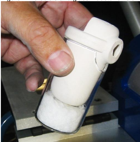
Figure 17: crucible and glass inductor shield
