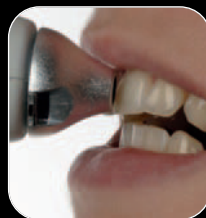
Incorrect positioning of the tooth - instrument tilted away from tooth allowing ambient light into measurement
