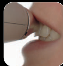
Incorrect positioning of the tooth - instrument tilted away from tooth allowing ambient light into measurement
