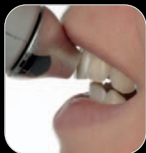
Incorrect positioning of the tooth - instrument tilted away from tooth allowing ambient light into measurement
