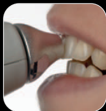
Incorrect positioning of the tooth - instrument tilted away from tooth allowing ambient light into measurement
