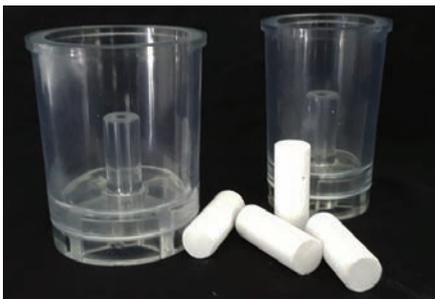
Low-wear, easy-to-clean silicone investment rings for pressed ceramics. The separation from the muffle is simplified by the cone shape. The transparent PVC allows to recognize the exact placement of the wax crowns as well as a perfect inflow of the investment material.
